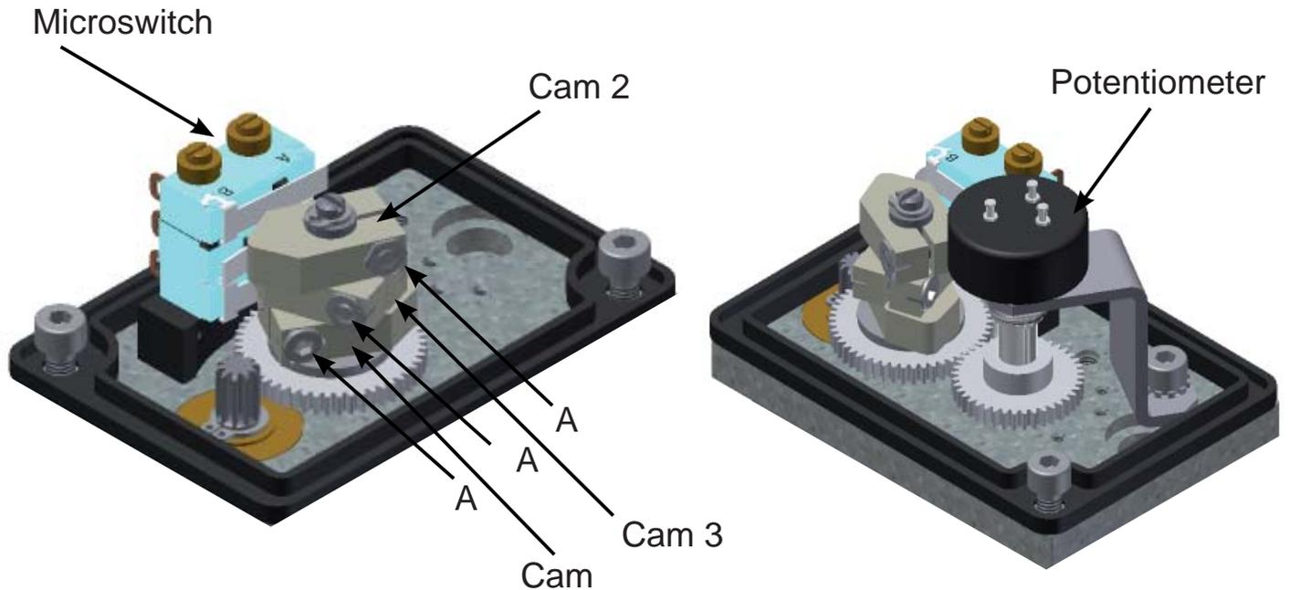
To adjust the stroke of the Push Tube to the set value, turn on the Cams 1 and 2 as follows:
