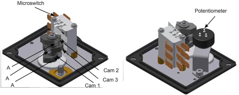
To adjust the stroke of the Push Tube to the set value, turn on the Cams 1 and 2 as follows:
