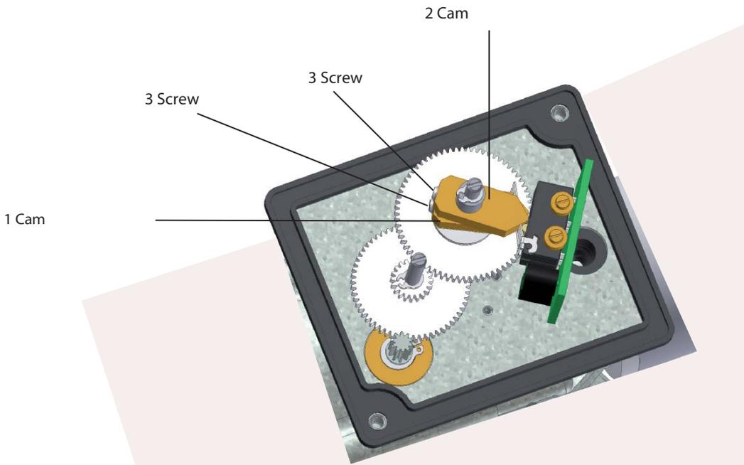
To adjust the stroke of the Push Tube to the set value, turn on the Cams 1 and 2 as follows:
